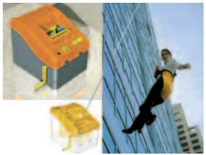
The Spider is designated for multi self-rescue from high-rise buildings. It can be permanently installed on the floor or on a wall and is always ready for immediate use. The occupant puts on a harness, attaches himor herself to the descent cable, and then exits the building. The device automatically controls the descent at a safe velocity. A redundant friction brake provides additional safety.
