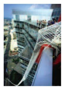
The Baker Life Chute is a self-contained unit that can be stored inside or on top of a structure and can be moved by hand to the safest exit locations, including windows, balconies, or roofs. It is triggered by the fire alarm and unfolds automatically from the structure; escape is accomplished by sliding down the chute, slowing as appropriate by outward pressure of feet and with hands held above the head.
