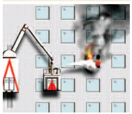
The automatic rescue climber comprises a device having a crane component and monorail elevator component for extending an arm to a desired location on the building. The elevator component incorporates a telescopic pole for adjusting the distance to a cabin on the other end of the pole. The cabin can be used for lifting firefighting and rescue personnel into the building and to evacuate occupants from the building to ground level.
